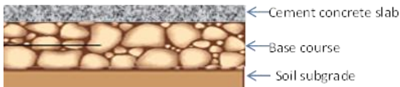
Figure 1.7 Components of rigid pavement in India
